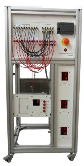
3-floor elevator traing set is designed as a sample for electromechanical control and PLC applicaitons. Its transparent structure is preferred to examine the electrical connections and mechanical parts. 45x45 anodized aluminum sigma profile is used in the construction of the set.
