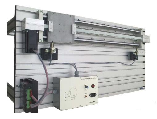
The set consists of a stepper motor and driver is designed to manipulate the speed and position controls.
