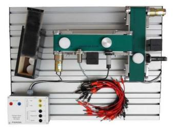
The 2 axes conveyor bant training set designed as a sample for the conveyors used in industrial systems and product classification lies on the aluminium sigma profile platform.
