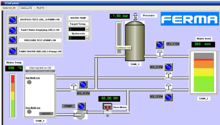
There are also online watch windows, and graphic drawing properties, variables (Pressure, level, temperature, flow) versus time.
