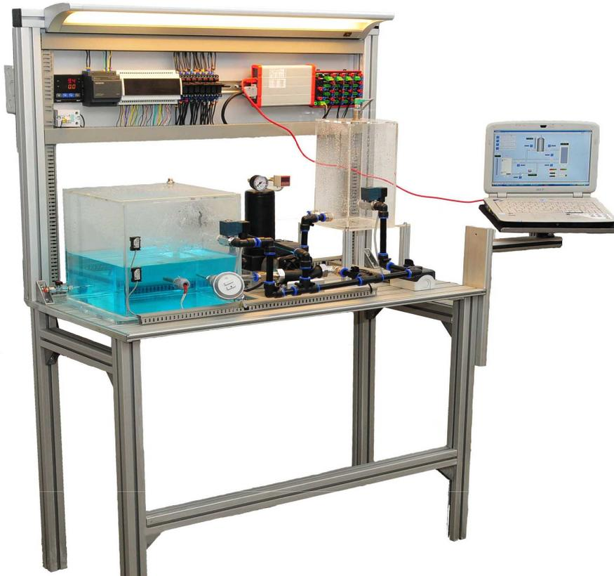
The process automation training set allows the learner to enable different flows from the main tank to others and back. The learner can change the temperature, pressure and the flow of the fluid. The control is done through a PC connected to the system. The learner can observe in realtime what happens when the setup is changed. Moreover, the process is recorded at the same time through data acquisition on the PC.
