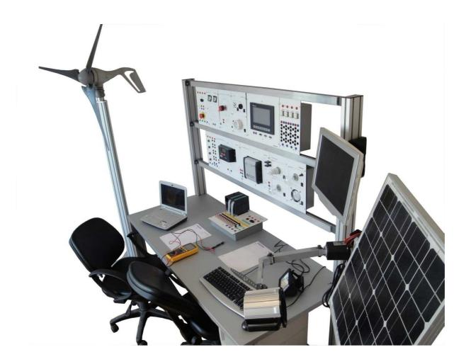
Renewable energy systems training set is designed to investigate the electricity generation with small wind turbines and solar panels. The set is a hybrid module available indoor use.
